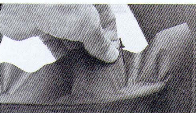
8 Wing tip – heat wrinkles (circled) and stretch Solartex in arrow direction
